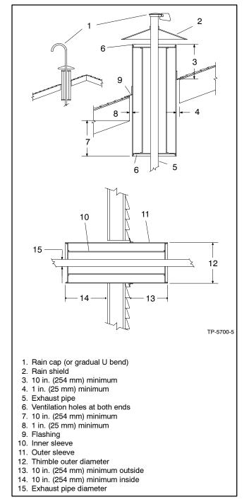
Figure 5-4 Double-Sleeved Thimbles and Rain Cap
